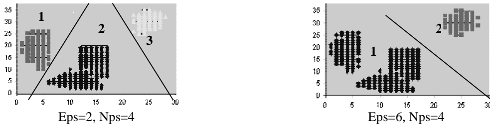
Figure 1: The different partitions resulting from running DBSCAN with different input parameter values.
